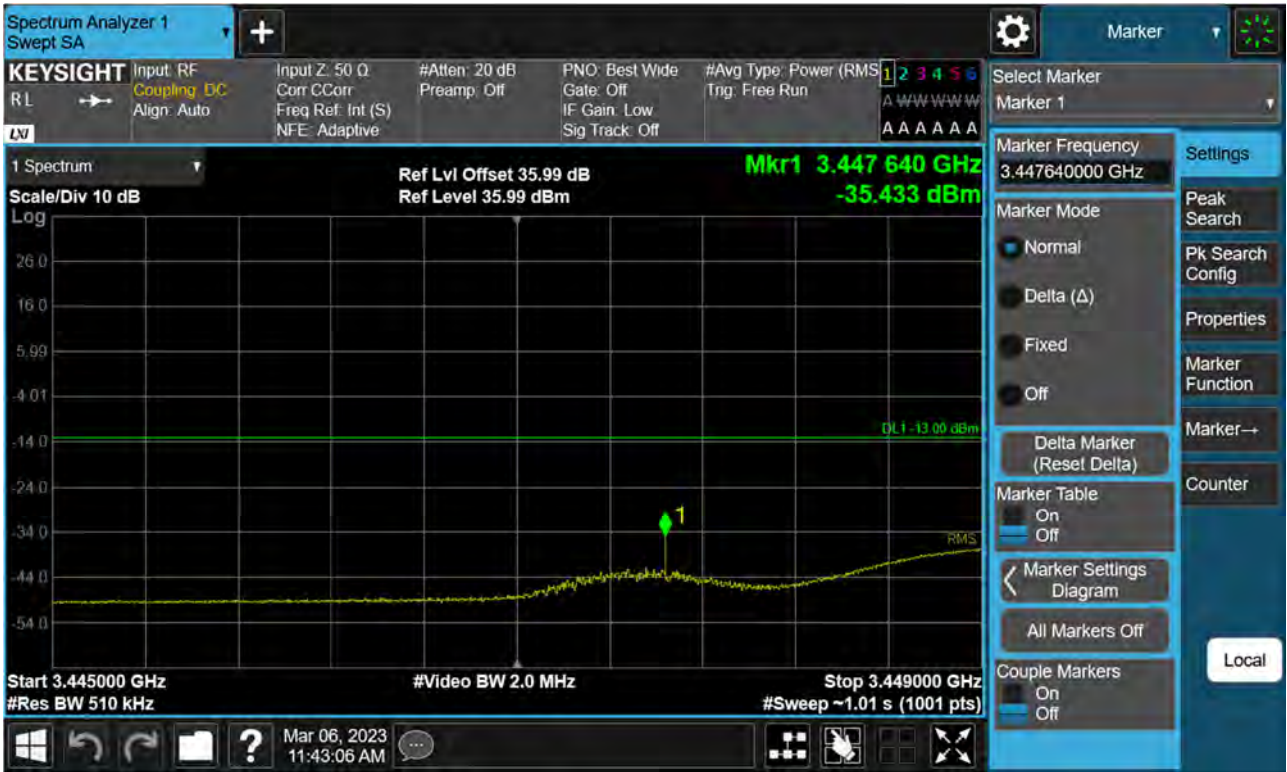
Sub6 n77(78). Low Band Edge Plot (20 M BW Ch.630668 BPSK 1RB)(2)
