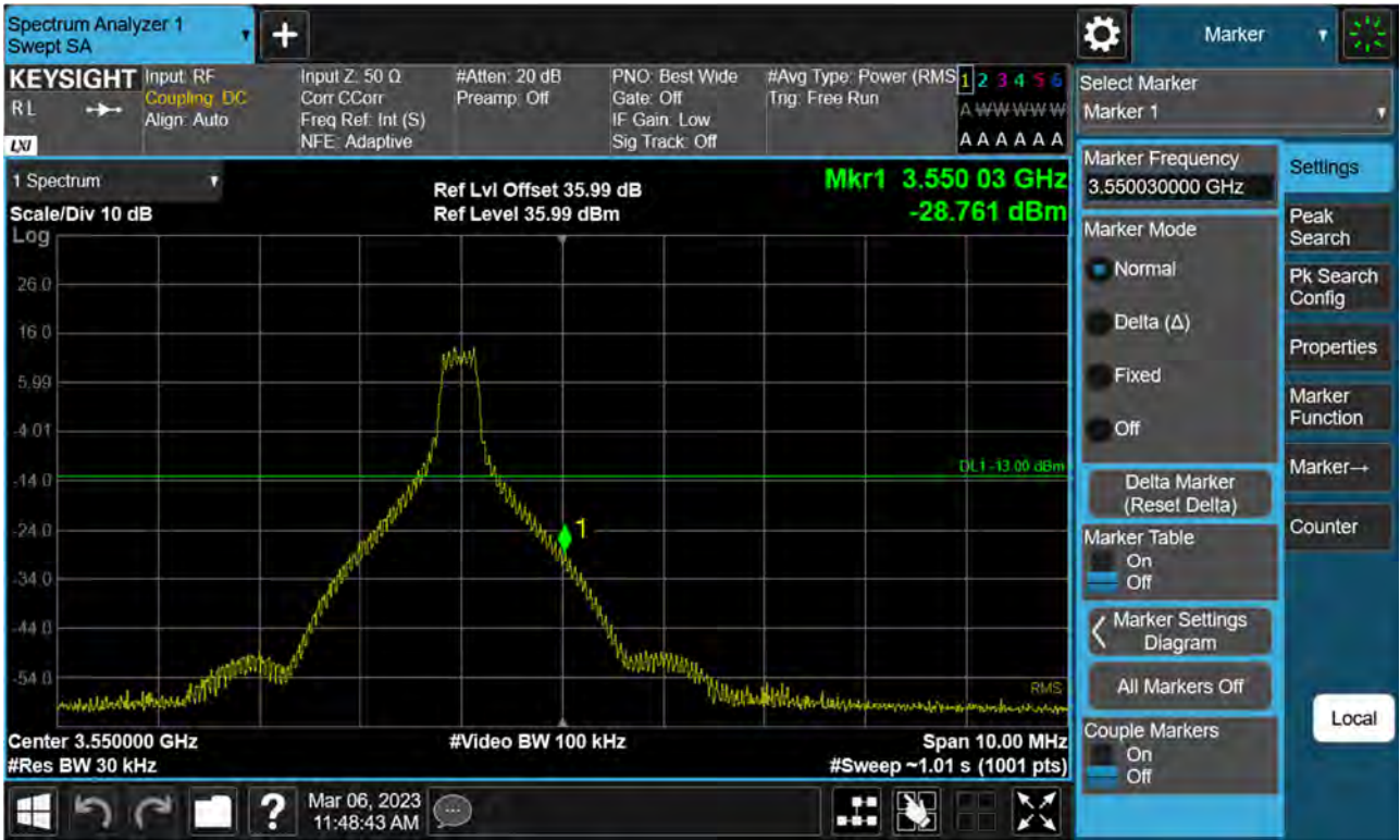
Sub6 n77(78). High Band Edge Plot (20 M BW Ch.636000 BPSK 1RB)(1)
