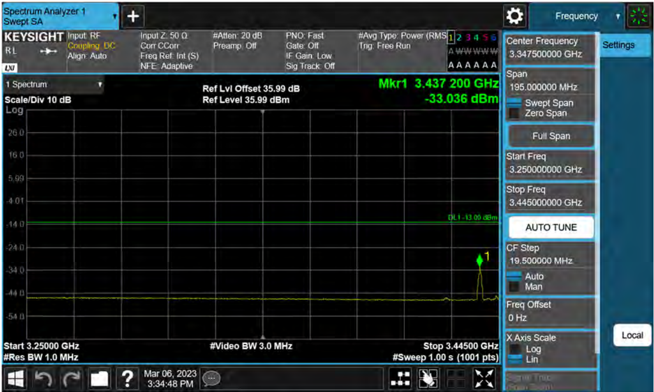
Sub6 n77(78). Low Band Edge Plot (30 M BW Ch.631000 BPSK 1RB)(3)
