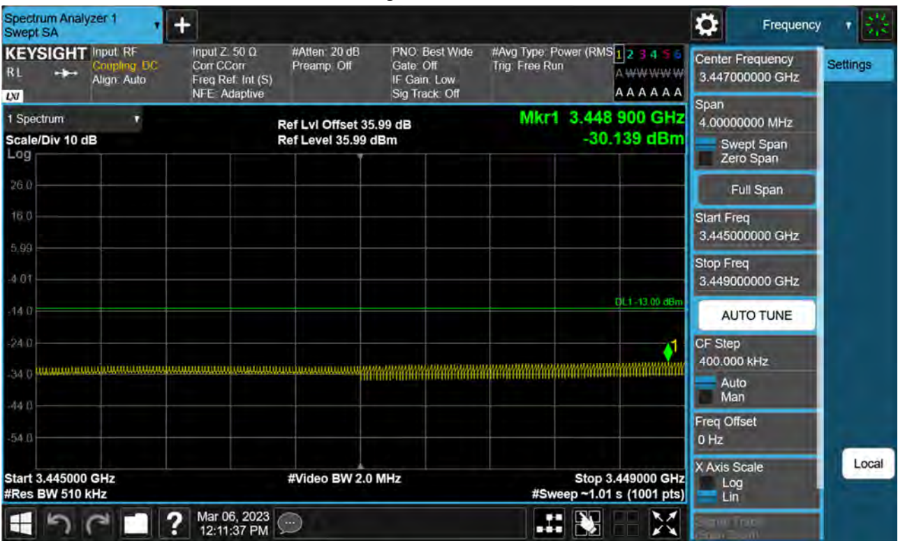
Sub6 n77(78). Low Band Edge Plot (40 M BW Ch.631334 BPSK FullRB)(2)
