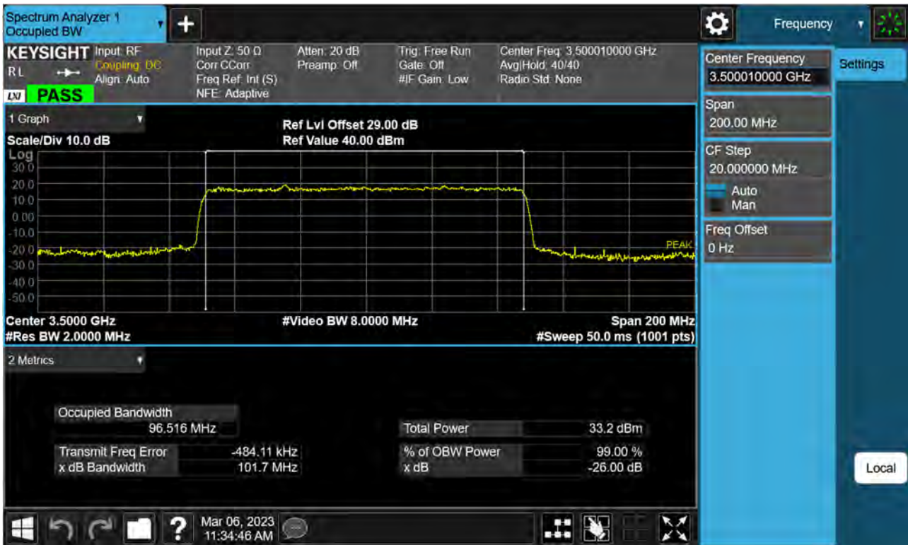
Sub6 n77(78). Occupied Bandwidth Plot (100 M BW Ch.633334 BPSK)
