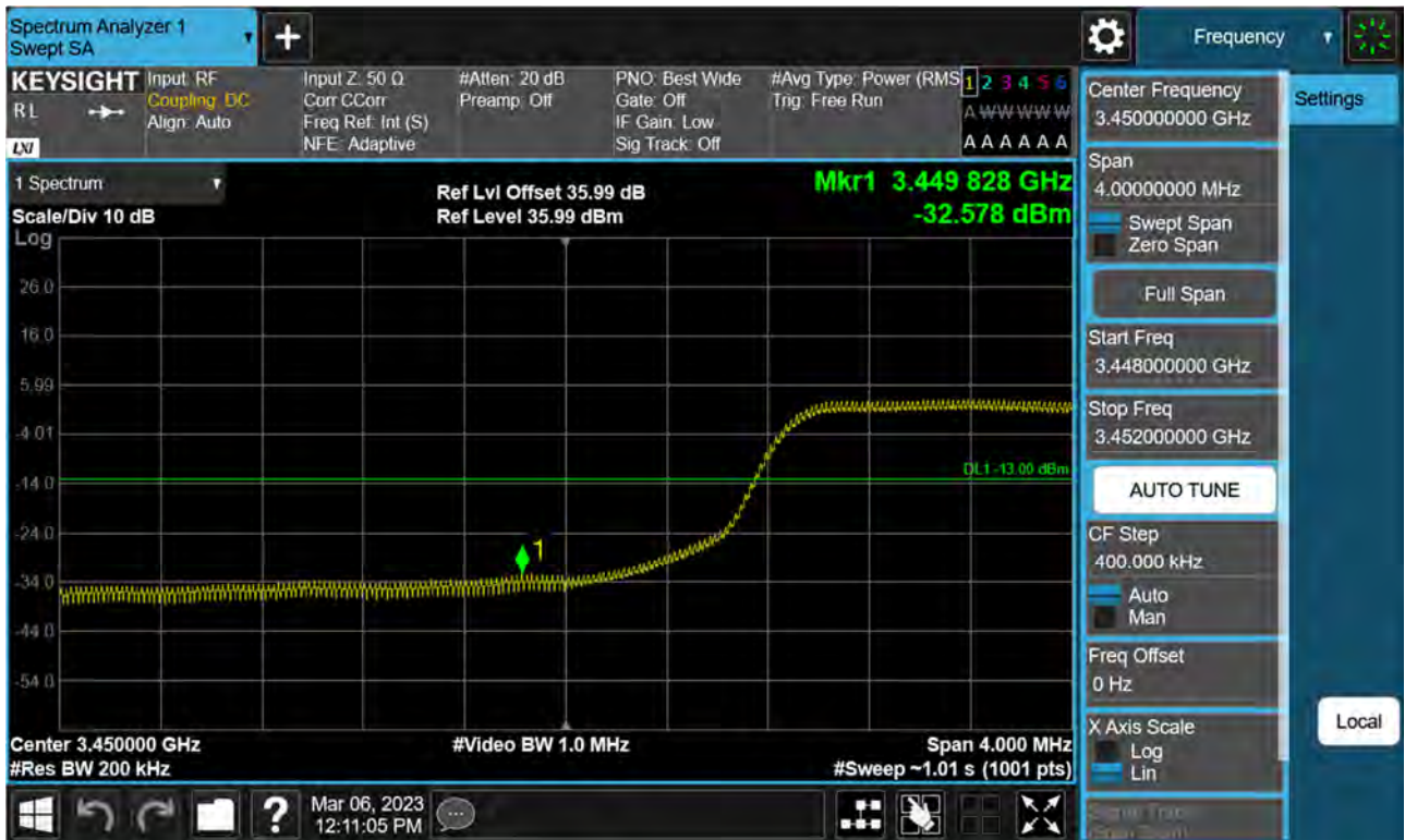
Sub6 n77(78). Low Band Edge Plot (40 M BW Ch.631334 BPSK FullRB)(1)
