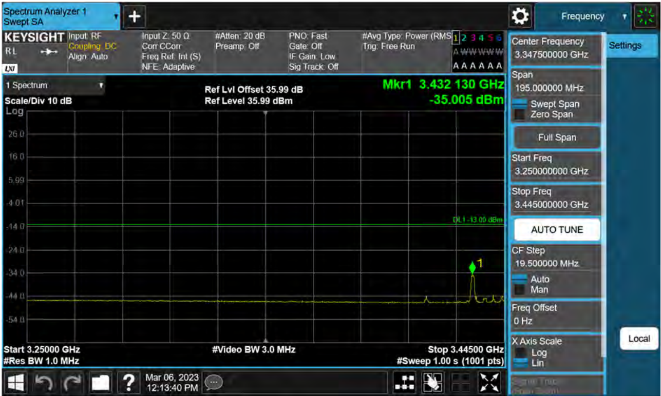
Sub6 n77(78). Low Band Edge Plot (40 M BW Ch.631334 BPSK 1RB)(3)
