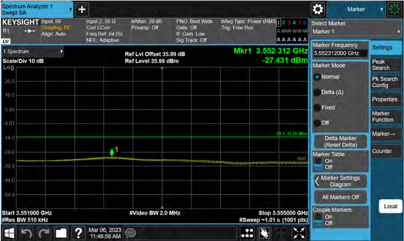
Sub6 n77(78). High Band Edge Plot (20 M BW Ch.636000 BPSK FullRB)(2)
