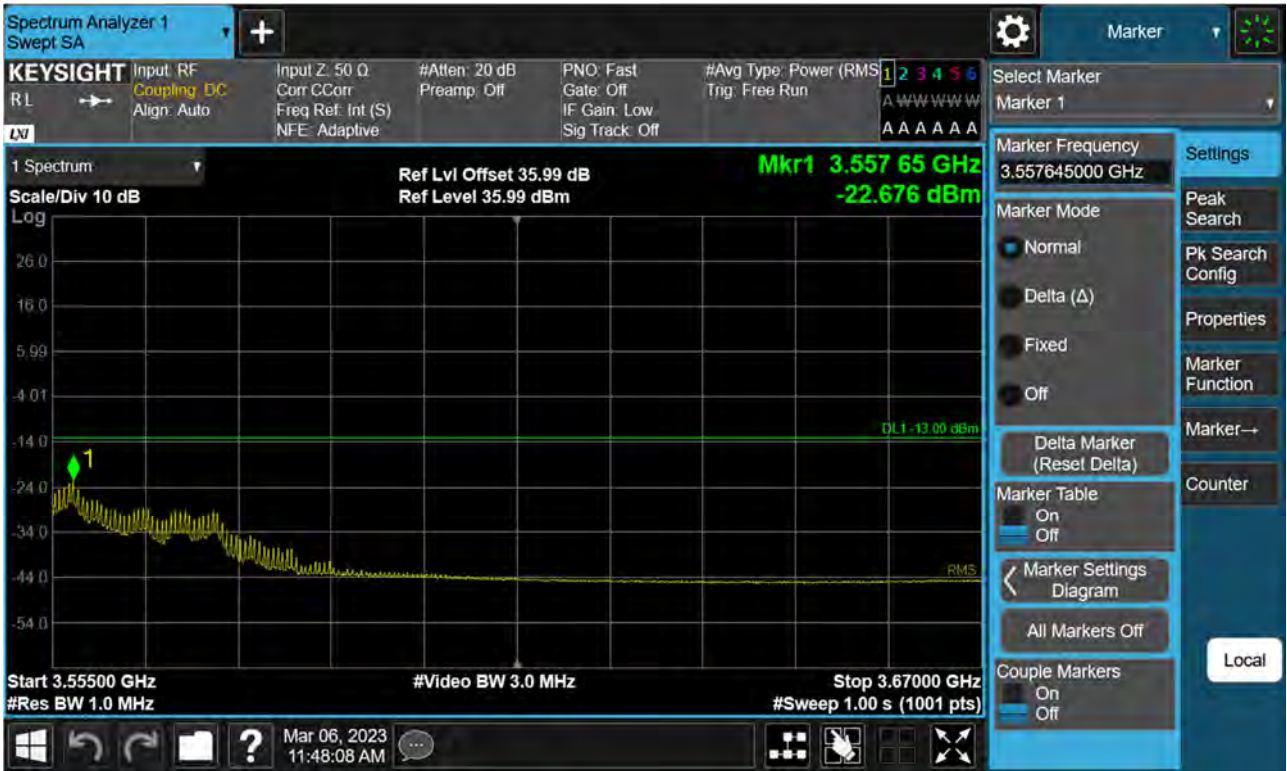
Sub6 n77(78). High Band Edge Plot (20 M BW Ch.636000 BPSK FullRB)(3)
