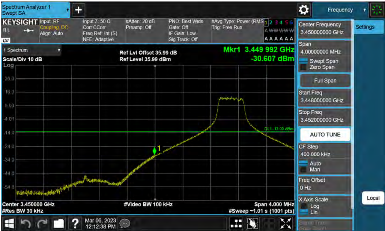
Sub6 n77(78). Low Band Edge Plot (40 M BW Ch.631334 BPSK 1RB)(1)
