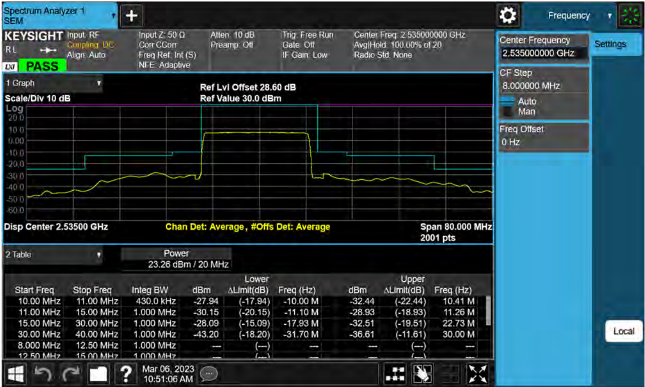
Sub6 n7. Mid Channel Edge Plot (20 MHz Ch.507000 BPSK)
