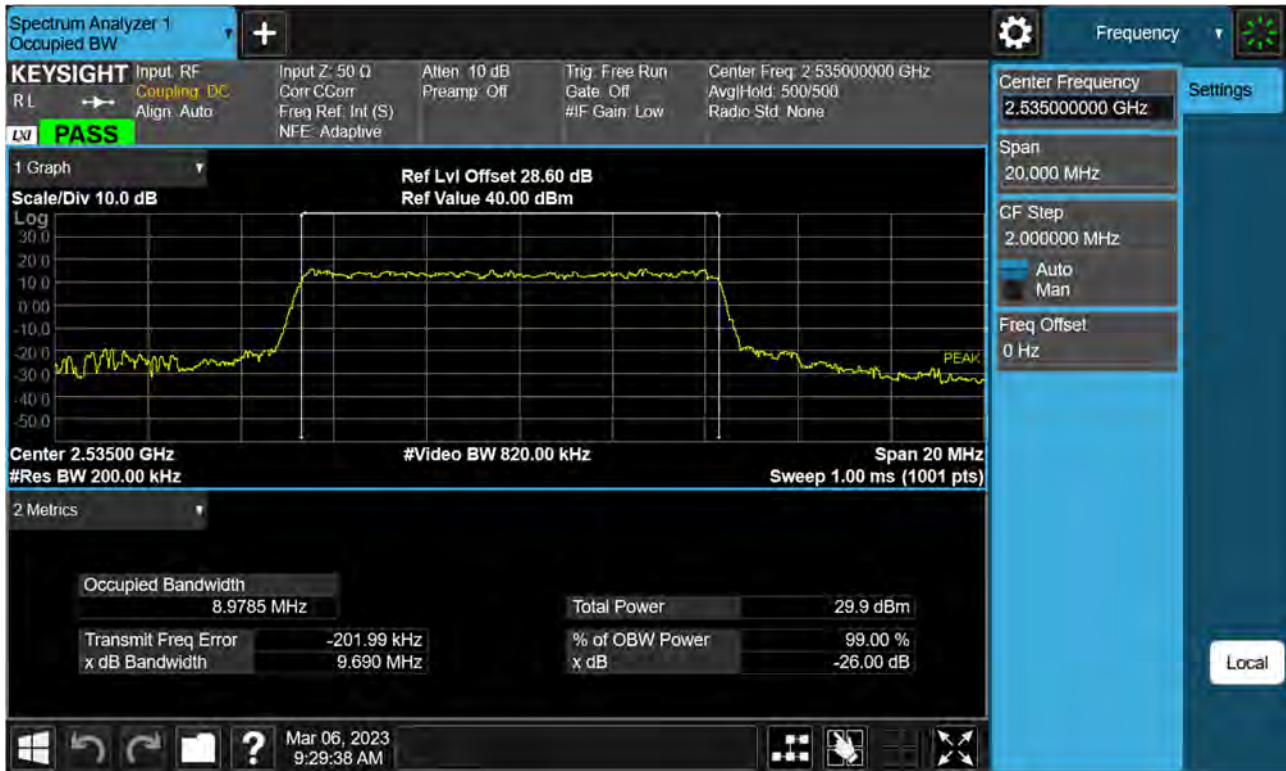
Sub6 n7. Occupied Bandwidth Plot (10 M BW Ch.507000 16QAM)
