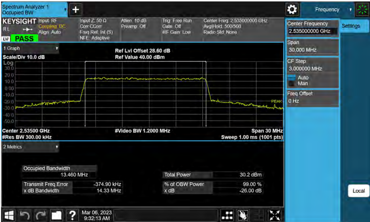
Sub6 n7. Occupied Bandwidth Plot (15 M BW Ch.507000 16QAM)
