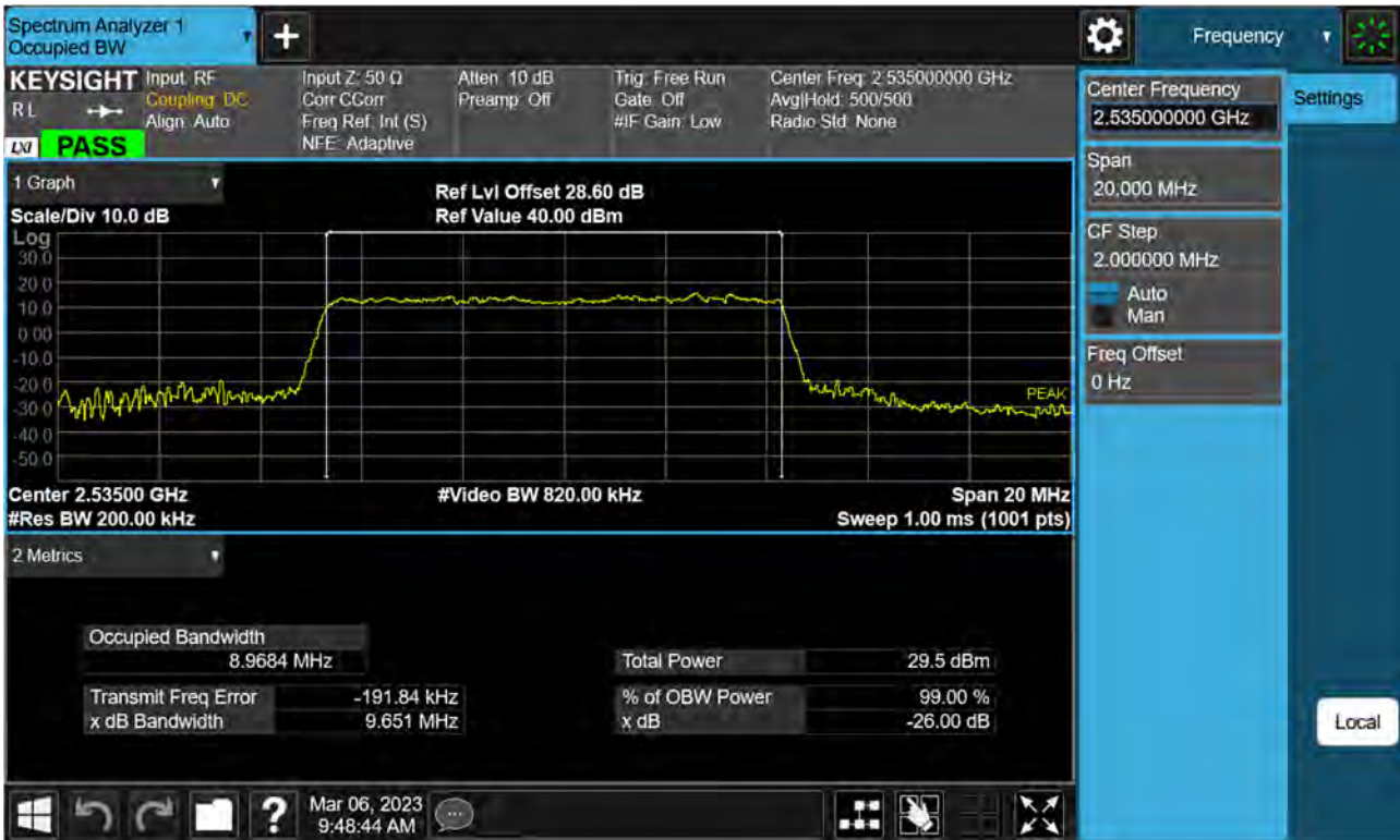
Sub6 n7. Occupied Bandwidth Plot (10 M BW Ch.507000 64QAM)
