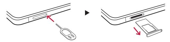
2 Put the memory card on the memory card tray and insert the tray into the device in the direction shown below.
