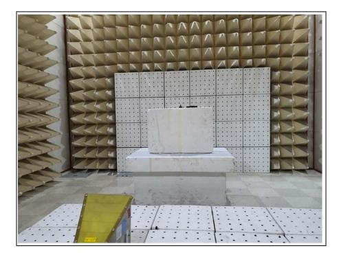
4. Photo of Radiated Spurious Emission Test (Above 1 🖽)\_WWAN
