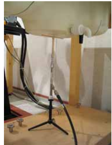
Photo of the dipole Antenna
