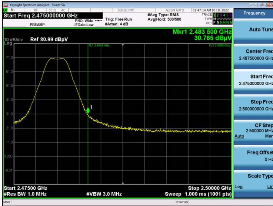
Radiated Restricted Band Edges plot – Average& Peak Result (CH.26: 2480 MHz)
