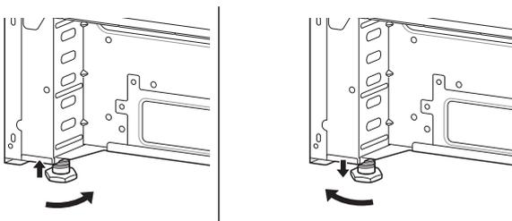
Use a level to check your adjustments. Place the level diagonally on the oven rack, and check each direction for level.
