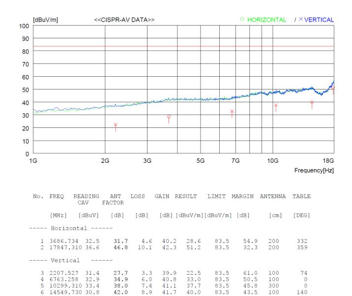
Result = Reading CISPR-Average + Antenna Factor + Loss - Gain
