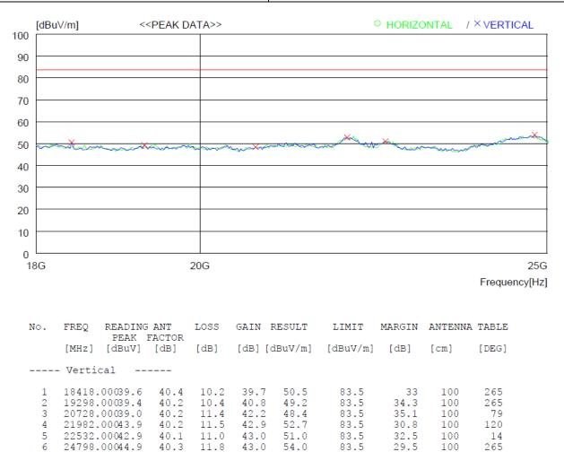
Result = Reading PEAK + Antenna Factor + Loss - Gain
