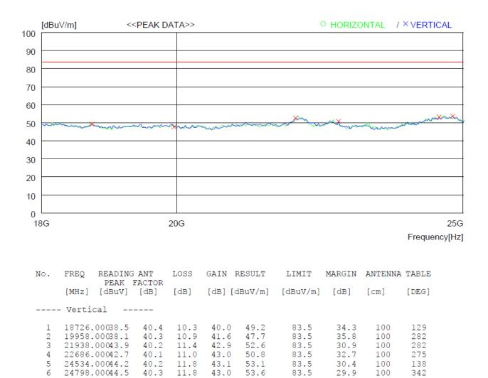
Result = Reading PEAK + Antenna Factor + Loss - Gain
