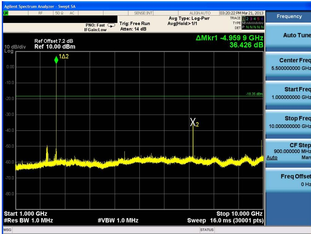
Test Plots (GFSK) - 10 GHz - 25 GHz (RBW:1 MHz, VBW: 1 MHz)
