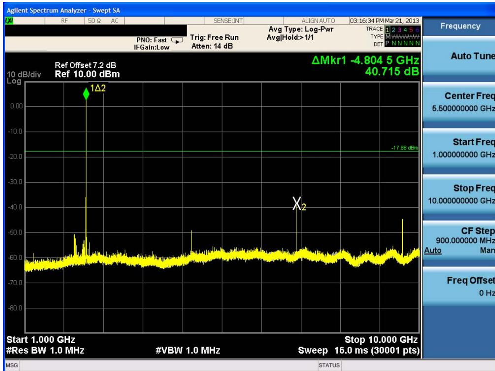
Test Plots (GFSK) - 1 GHz - 10 GHz (RBW:1 MHz, VBW: 1 MHz)
