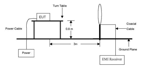
The diagram below shows the test setup that is utilized to make the measurements for emission from 30 Mb to 1 Gb.
