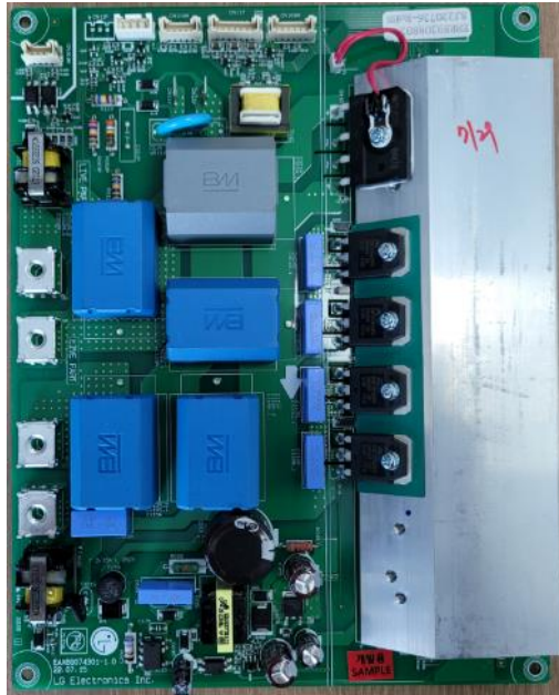
< Inverter 2B PCB (front) >
