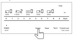
**3** To set and adjust the **Simmer Level**, touch the corresponding **Power Level**.
