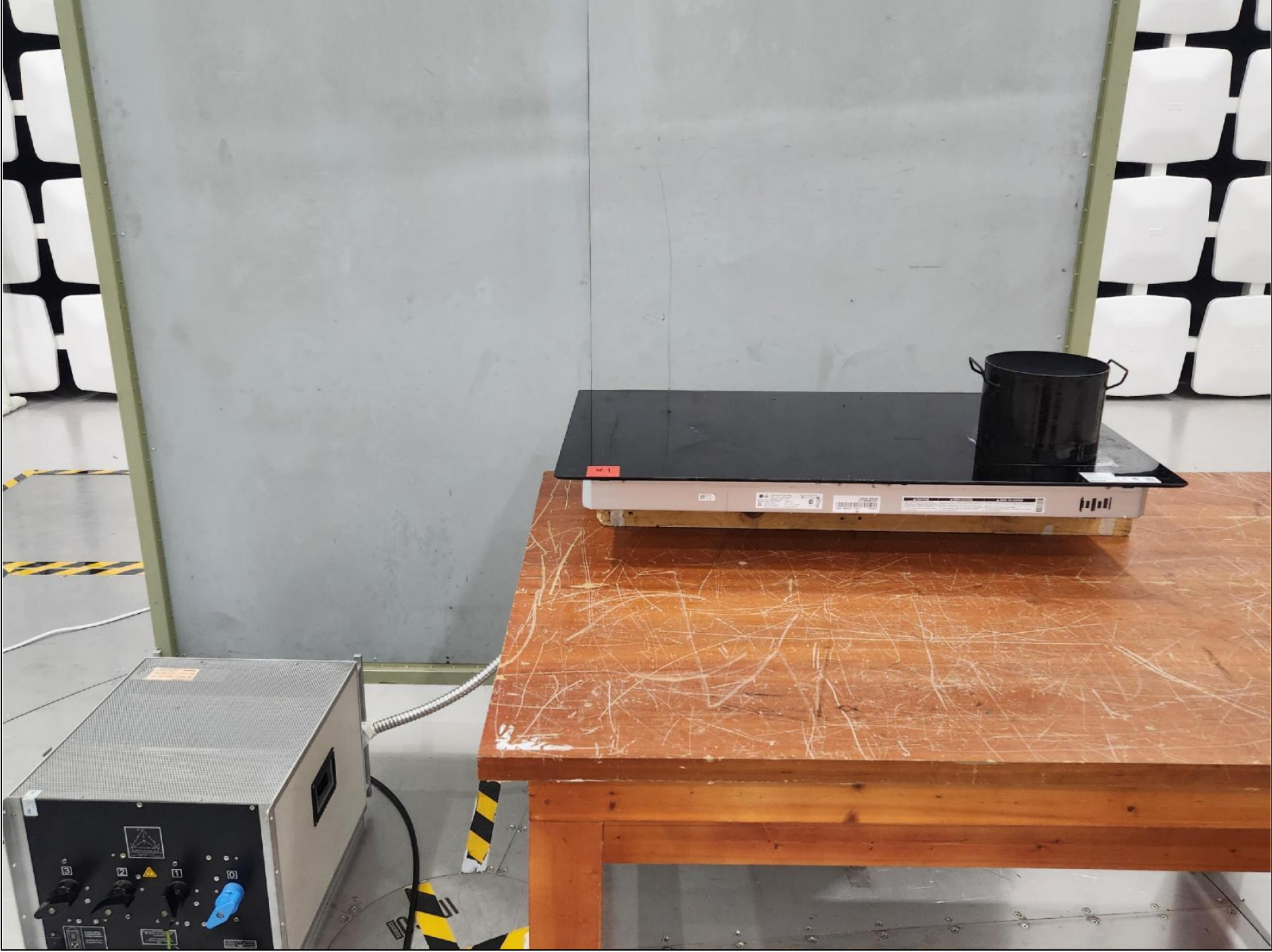
Continuous Conducted Emission at main _ Front
