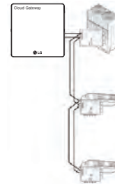
<Correct example : RS485 BUS format connection>
