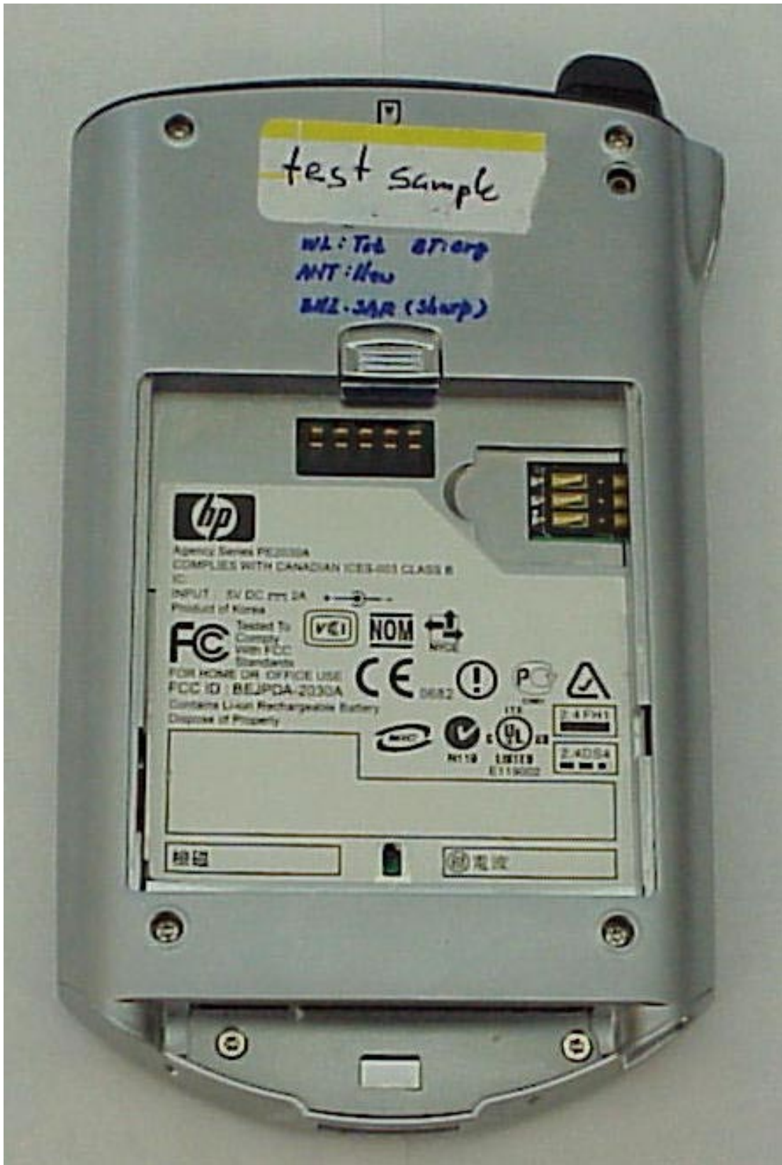
EUT Rear View with Label Placement
