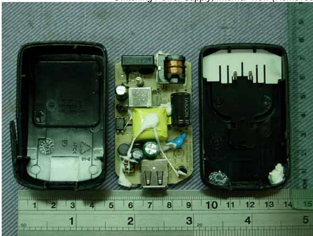
Figure 23 Switching Power Supply, Internal View (Removed Covers)
