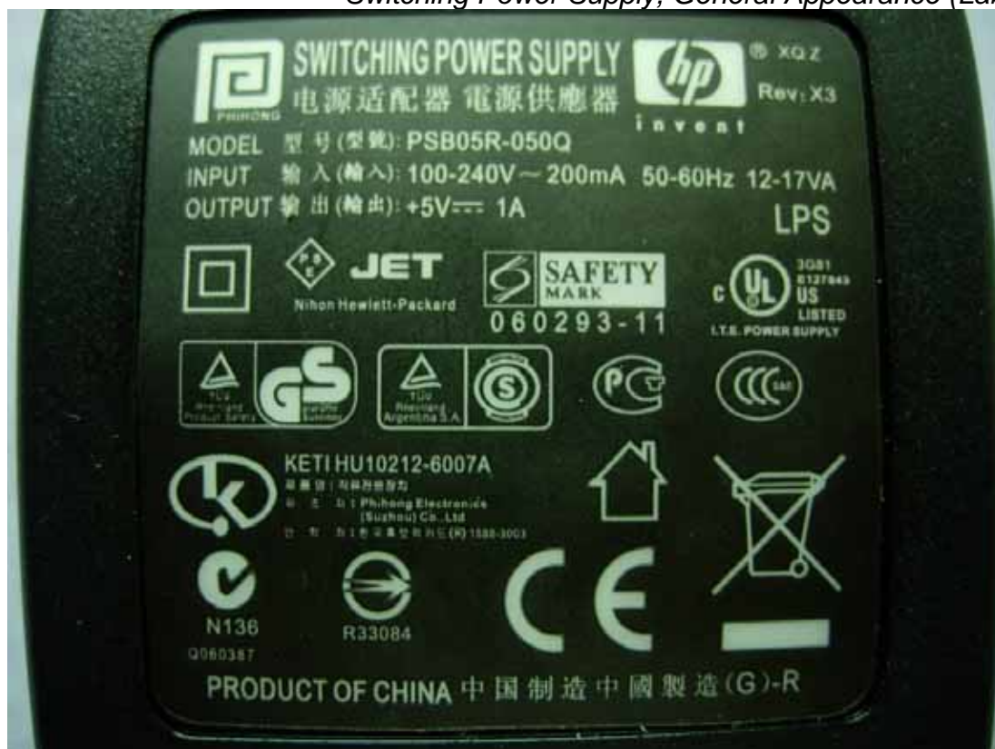
Figure 7 Switching Power Supply, General Appearance (Label View)
