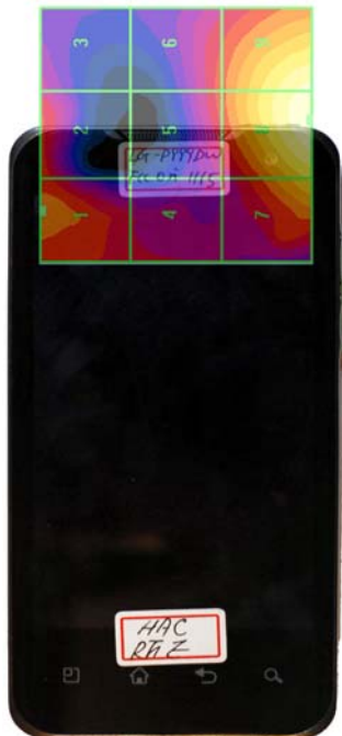
Figure 17-4 E-Field WD Scan overlay
