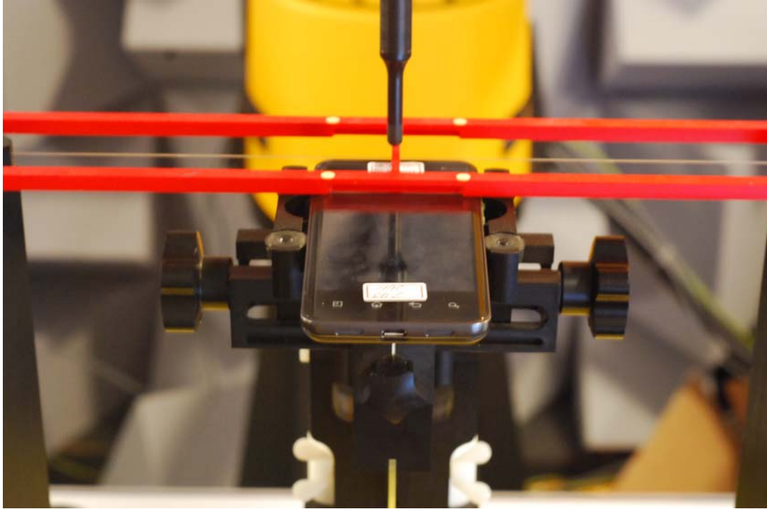
Figure 17-1 Ear Reference Point HAC Phantom Alignment
