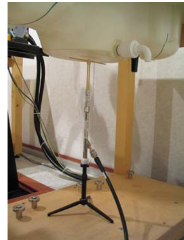
Photo of the dipole Antenna
