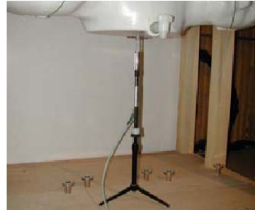
Figure 9.1 Dipole Verification Test Setup Diagram & Photo
