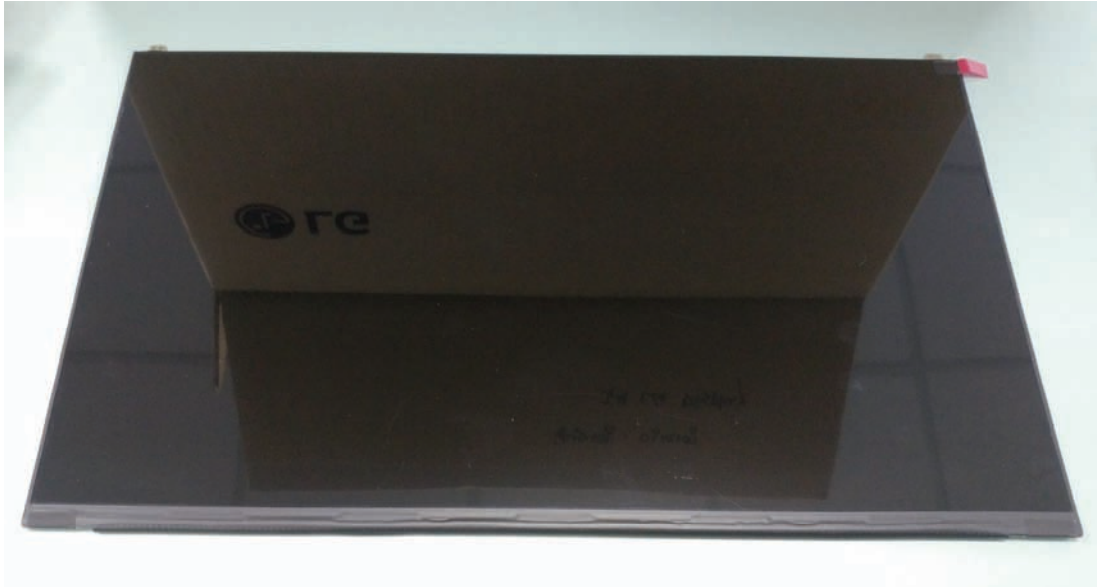
Figure 11 LG Display, M/N: LP156WFA(SP)(G1)/(AIT Including touch), LCD Panel, Front View
