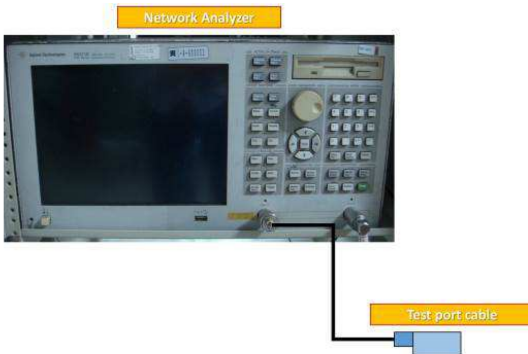
Figure 1. The schematic diagram for measuring VSWR
