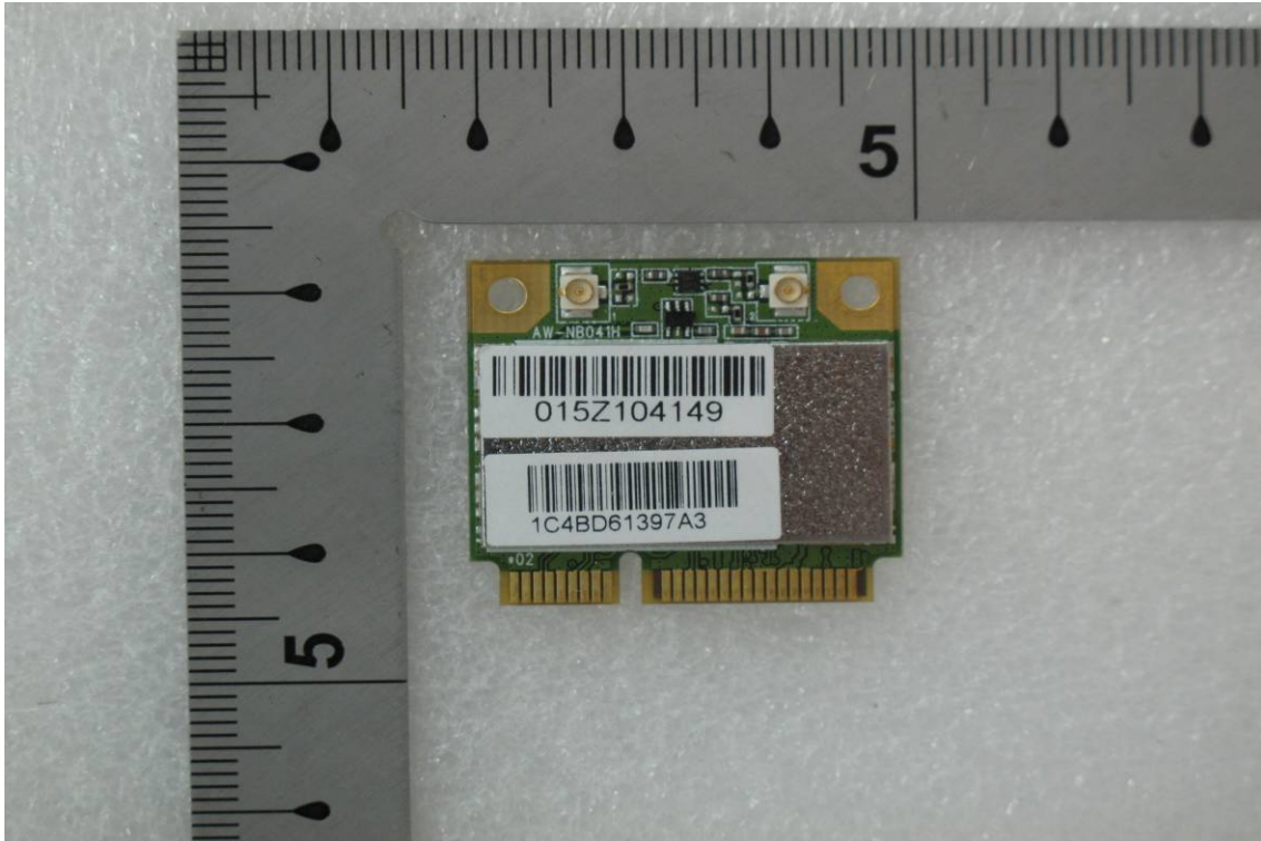
Internal View of EUT – 3 (WLAN /BT Module)
