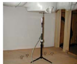
Figure 11.1 Dipole Verification Test Setup Diagram & Photo
