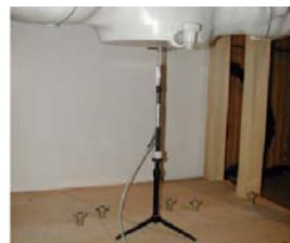
Figure 11.1 Dipole Verification Test Setup Diagram & Photo
