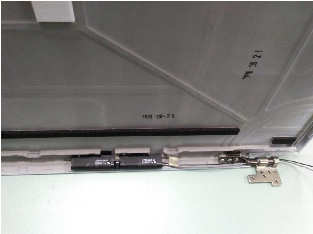
Figure 45 WLAN Antenna Position
