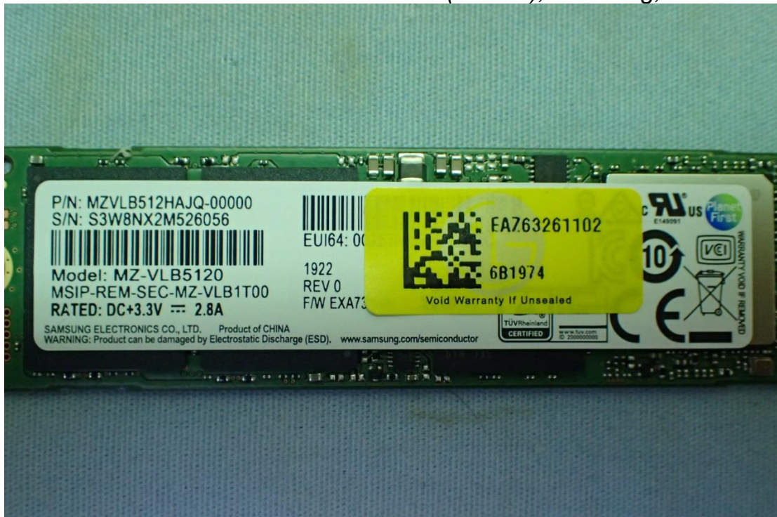
Figure 49 SSD (512GB), Samsung, Front View
