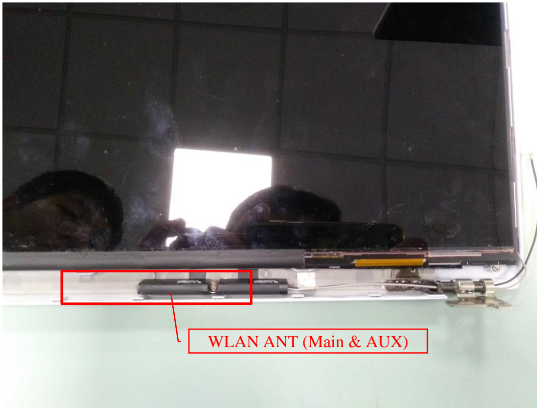
Figure 44 WLAN Antenna Position
