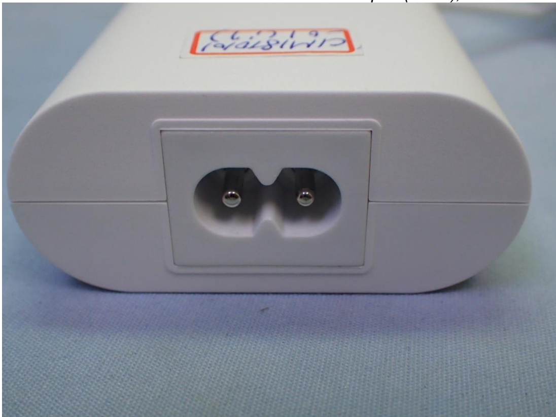
Figure 16 AC Adapter (White), AC Inlet View
