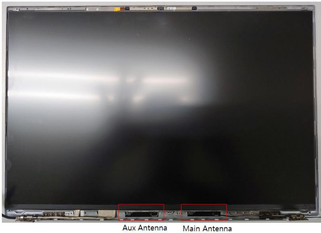
Figure 32 L1LRF009-CS-H, WLAN Combo Antenna Position
