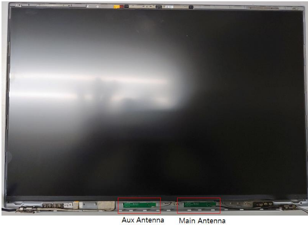
Figure 31 WA-P-LELE-04-011, WLAN Combo Antenna Position
