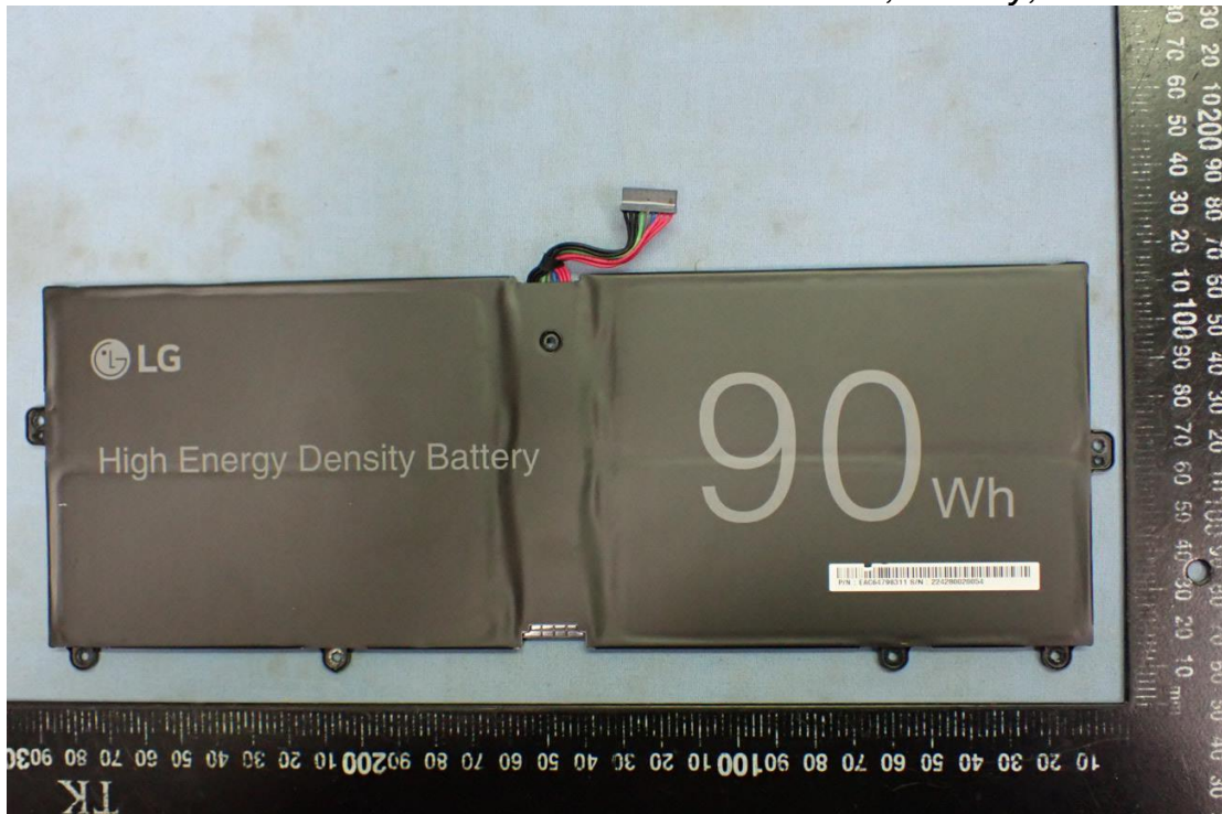
Figure 50 LBY122CM, Battery, Front View
