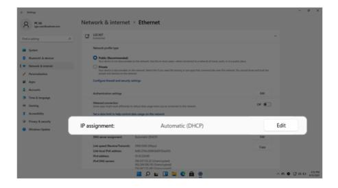
5 To use an automatic IP (DHCP), select [Automatic]. If you wish to use a static IP, set [Manual] > [IPv4] to [On] and enter the necessary item.
