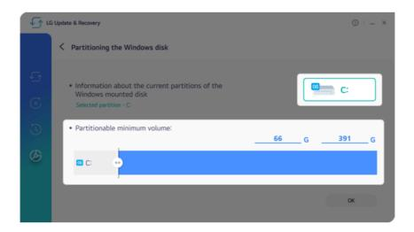
3 Set the capacity of the disk to be partitioned and select [OK].
