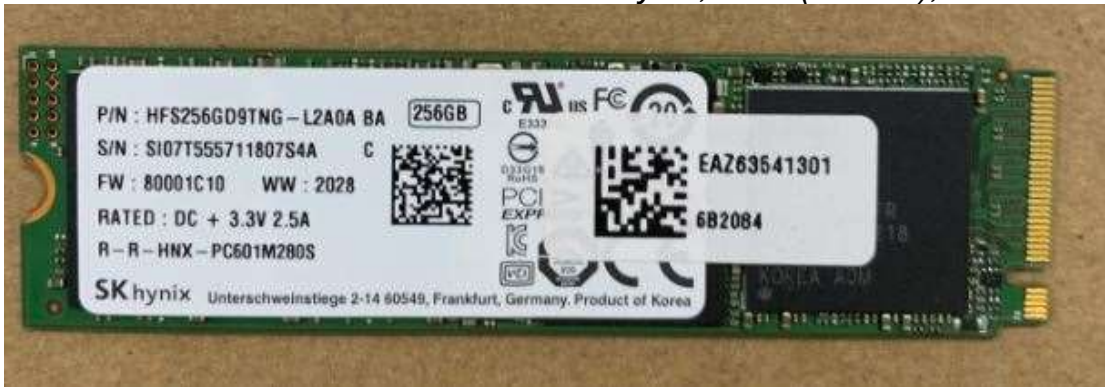
Figure 67 SK hynix, SSD (256GB), Front View
