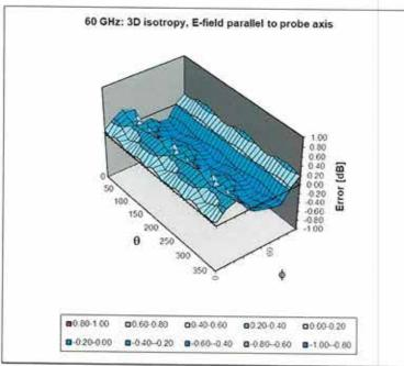
Probe isotropy for E<sub>tot</sub>: probe rotated  $\varphi = 0^{\circ}$  to 360°, tilted from field propagation direction  $\overline{k}$ Parallel to the field propagation ( $\psi = 0^{\circ} - 90^{\circ}$ ) at 30 GHz: deviation within ± 0.36 dB Parallel to the field propagation ( $\psi = 0^{\circ} - 90^{\circ}$ ) at 60 GHz: deviation within ± 0.37 dB
