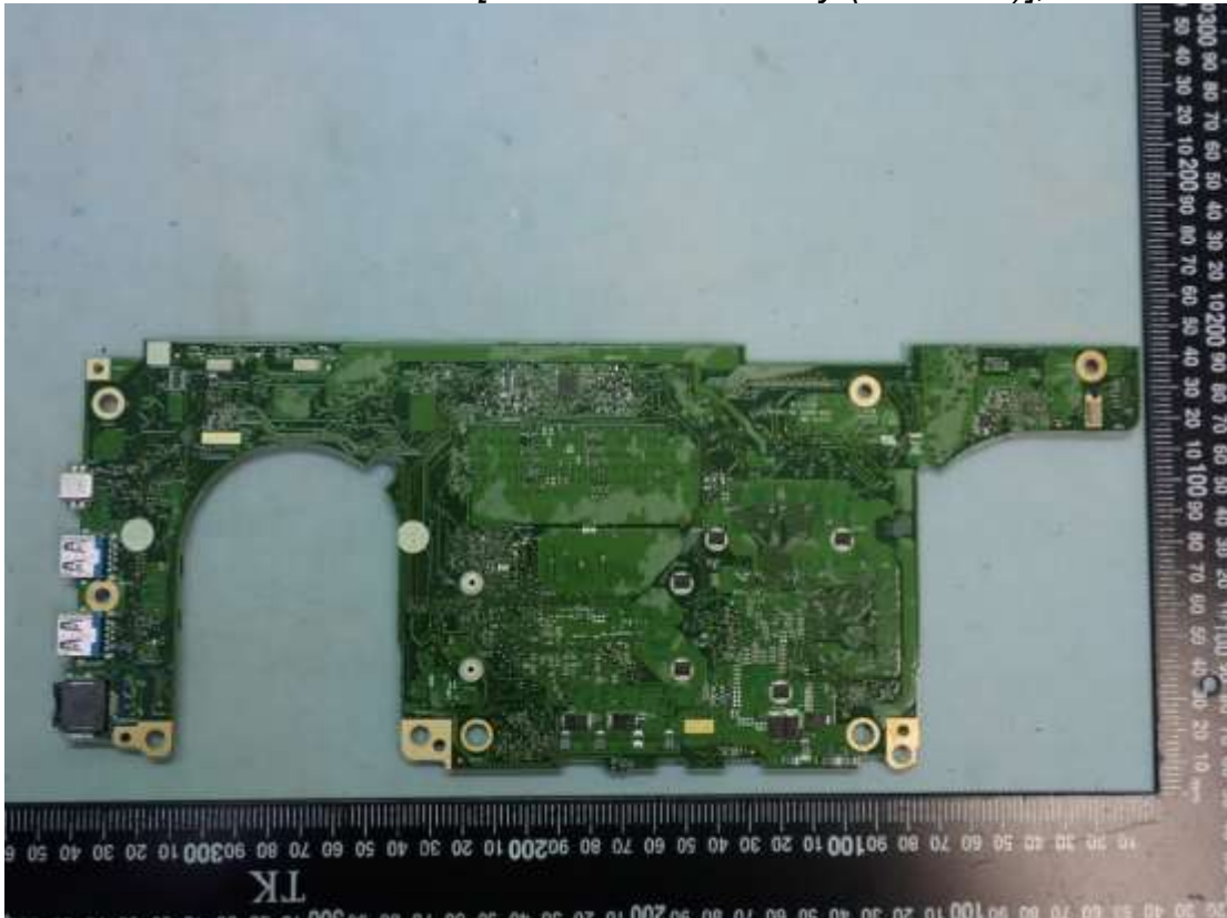
Figure 37 Main Board [with GPU & memory (on board)], Back View
