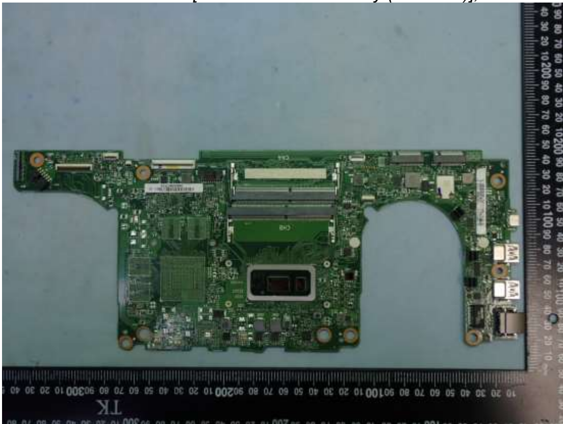
Figure 38 Main Board [without GPU & memory (on board)], Front View
