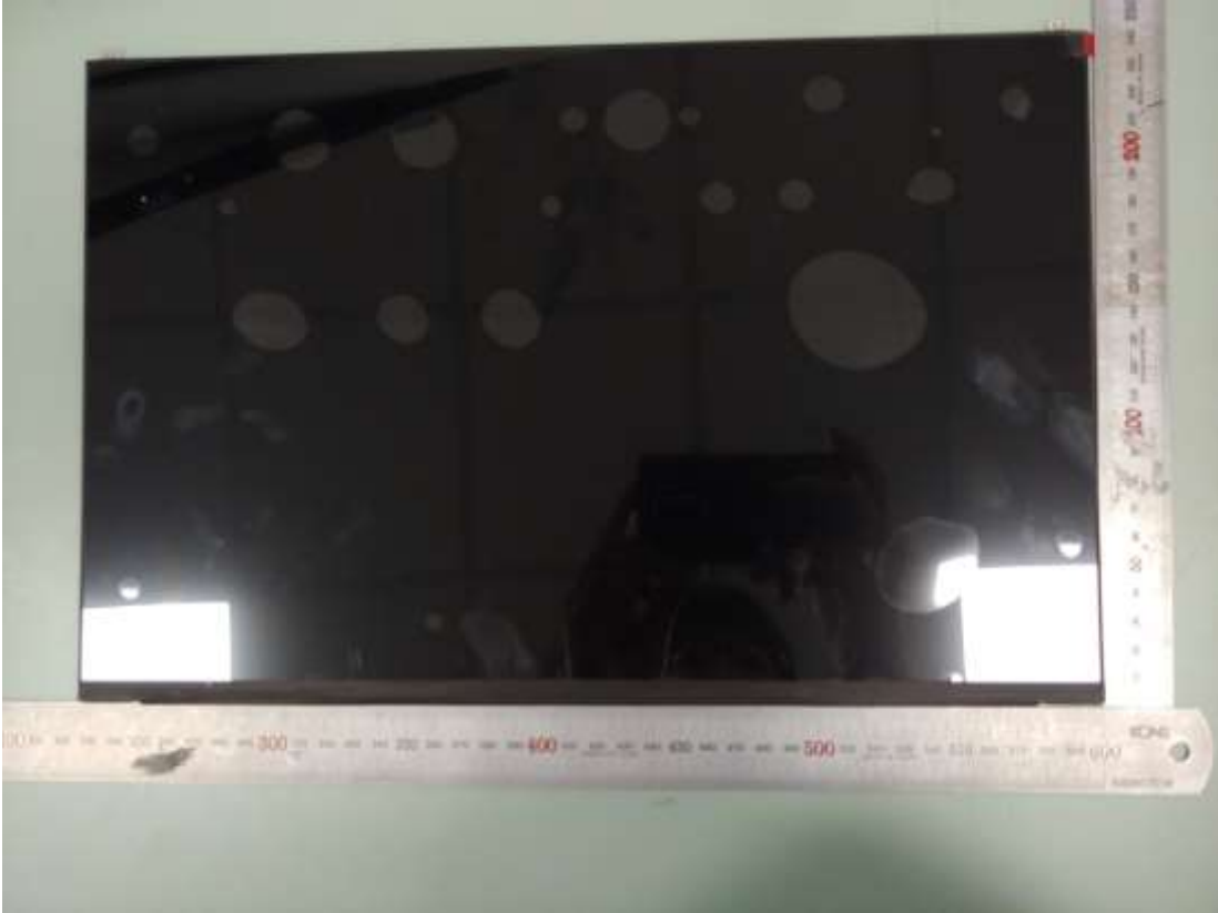
Figure 58 LGD, M/N LP170WQ1(SP)(A1), LCD Panel, Front View
