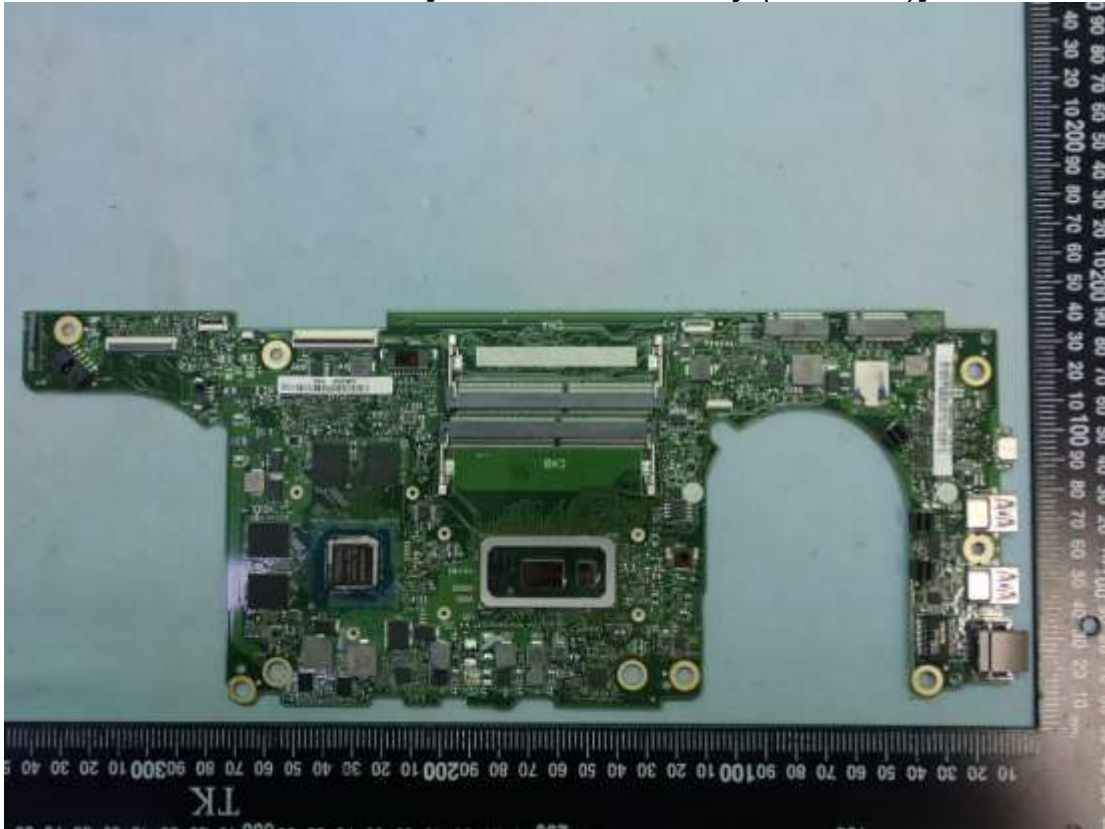
Figure 36 Main Board [with GPU & memory (on board)], Front View
