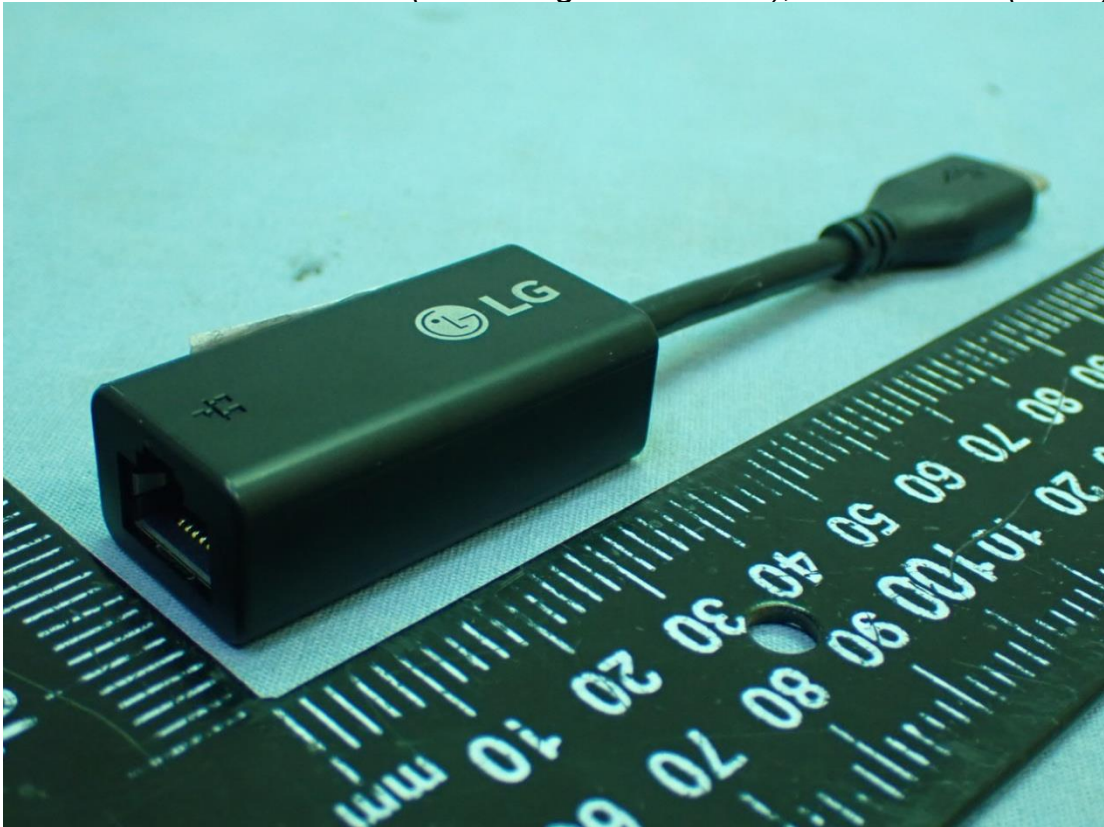
Figure 48 MEC (1000 Megabit Ethernet), LAN Gender (Black)
