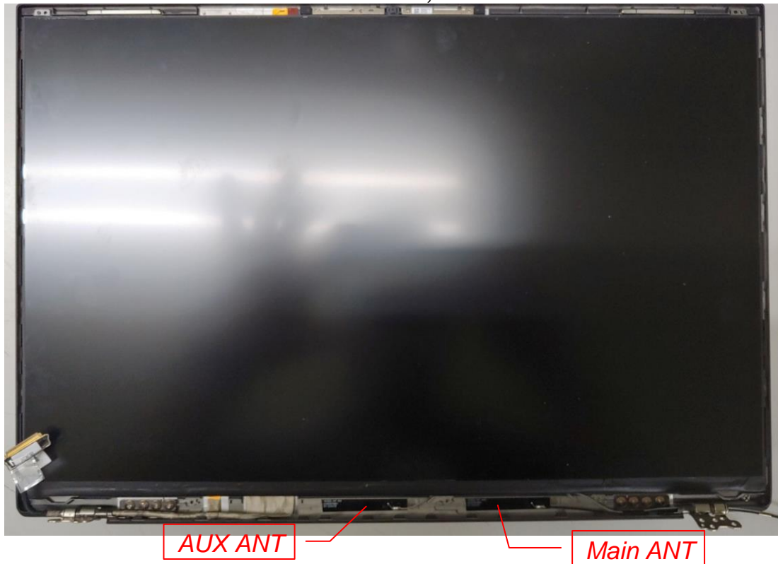
Figure 124 L1LRF008-CS-H, WLAN Combo Antenna Position
