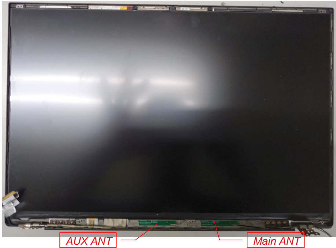
Figure 46 L1LRF008-CS-H, WLAN Combo Antenna Position
