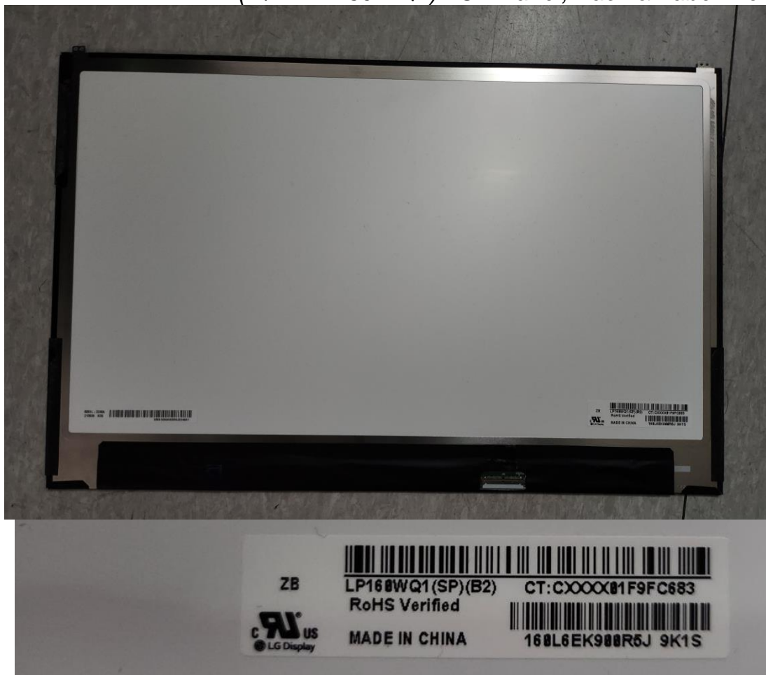
Figure 38 (M/N: LP160WQ1) LCD Panel, Back & Label View
