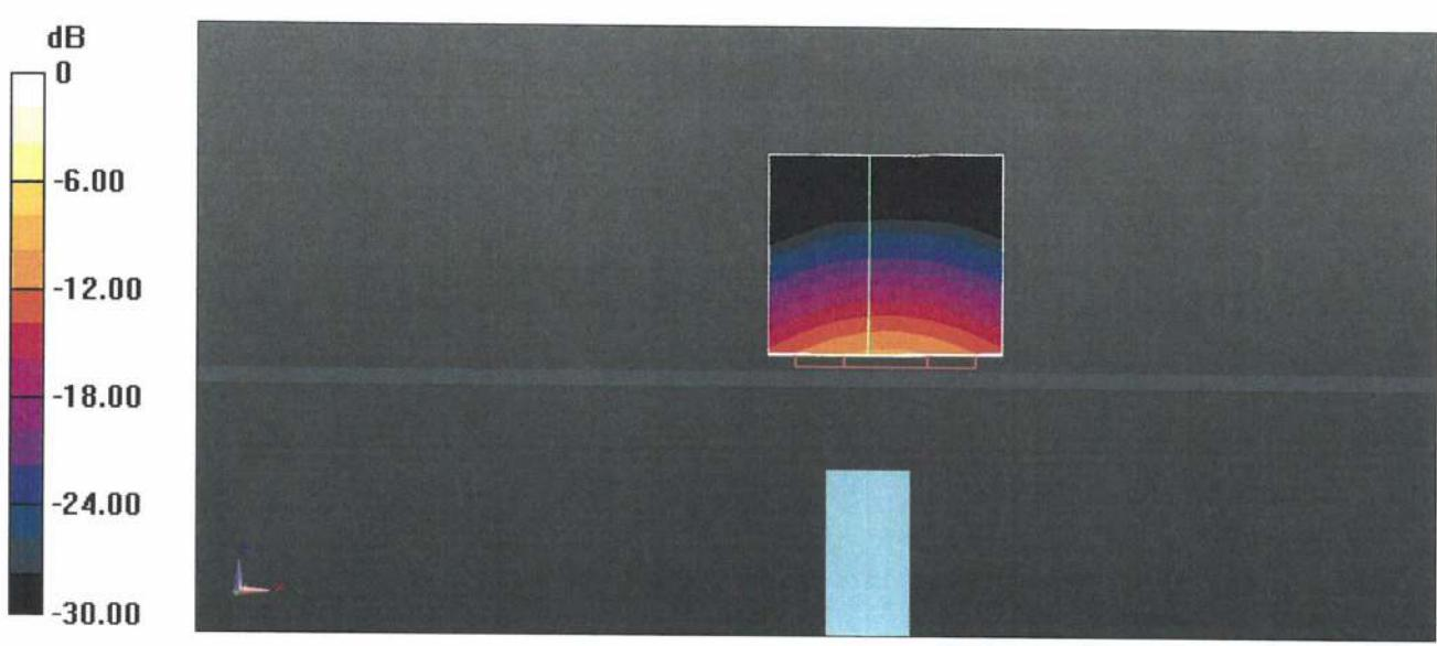
$$0 \text{ dB} = 18.0 \text{ W/kg} = 12.55 \text{ dBW/kg}$$
