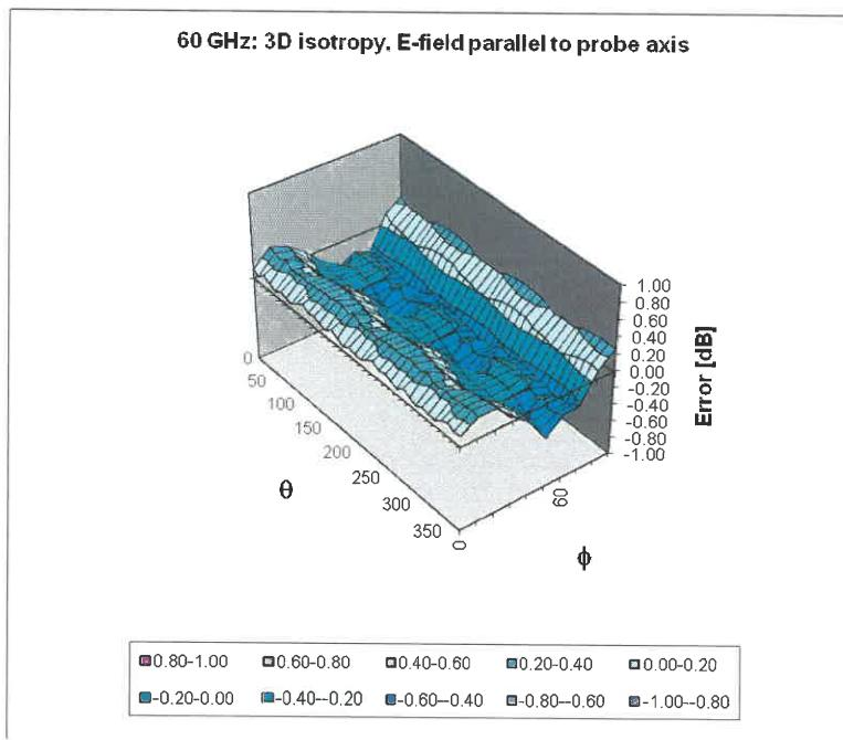
Probe isotropy for  $E_{\text{tot}}$ : probe rotated  $\varphi = 0^\circ$  to  $360^\circ$ , tilted from field propagation direction  $\hat{x}$
