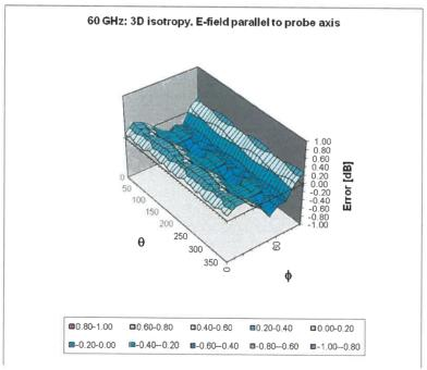
Probe isotropy for E<sub>tot</sub>: probe rotated  $\phi$  = 0° to 360°, tilted from field propagation direction  $\overline{k}$  Parallel to the field propagation ( $\psi$  =0° - 90°) at 30 GHz: deviation within ± 0.48 dB Parallel to the field propagation ( $\psi$  =0° - 90°) at 60 GHz: deviation within ± 0.35 dB
