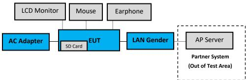
3.10.2. EUT Configuration for RF Conducted Test Items
