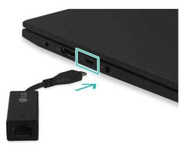
2 Connect the wired LAN cable to the LAN port.
