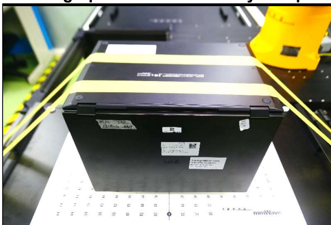
Bottom of Laptop Tested at 0 mm
