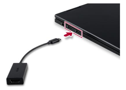
2 Connect the HDMI cable to the PC and the external device (TV, monitor) that supports HDMI.
