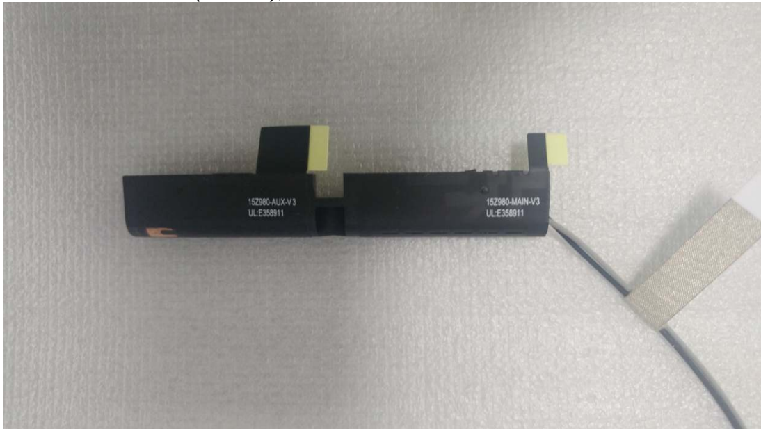
Figure 37 LG (INPAQ), M/N WA-F-LBLB-04-056 WLAN Combo Antenna
