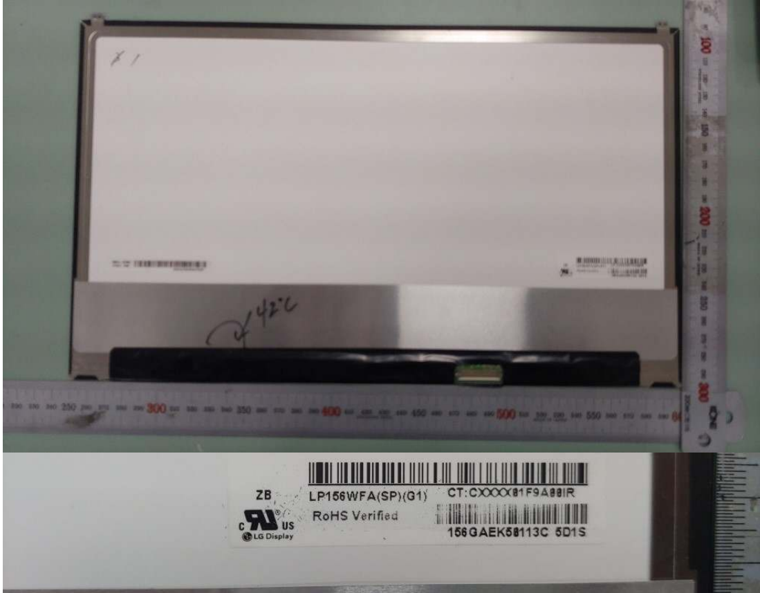
Figure 22 M/N: LP156WFA(SP)(G1)/( FHD IPS Touch), LCD Panel, Back/Label View
