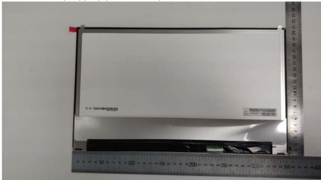
Figure 28 M/N: LP156WFD(SP)(Y1) (With Touch), LCD Panel, Back View/ Label View
