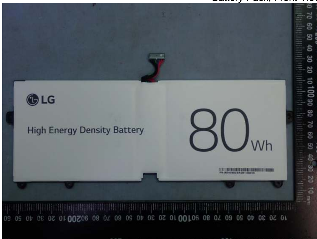
Figure 35 Battery Pack, Front View
