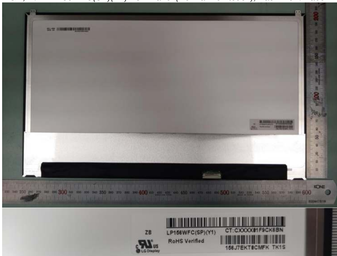
Figure 30 LGD, M/N LP156WFC(SP)(Y1) LCD Panel (Normal Non touch), Back View/ Label View
