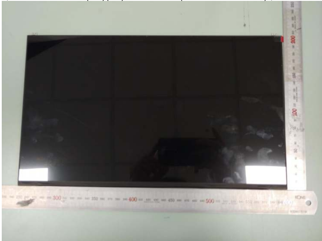
Figure 29 LGD, M/N LP156WFC(SP)(Y1) LCD Panel (Normal Non touch) , Front View
