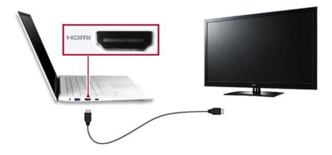
3 On the PC, press [Fn] + [F7] to display monitor (projector) toggling screen. Select the desired screen output.
