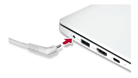
2 Open the LCD and check the charging state. When the AC adapter lamp is blinking, charge it fully with the AC adapter before using it.
