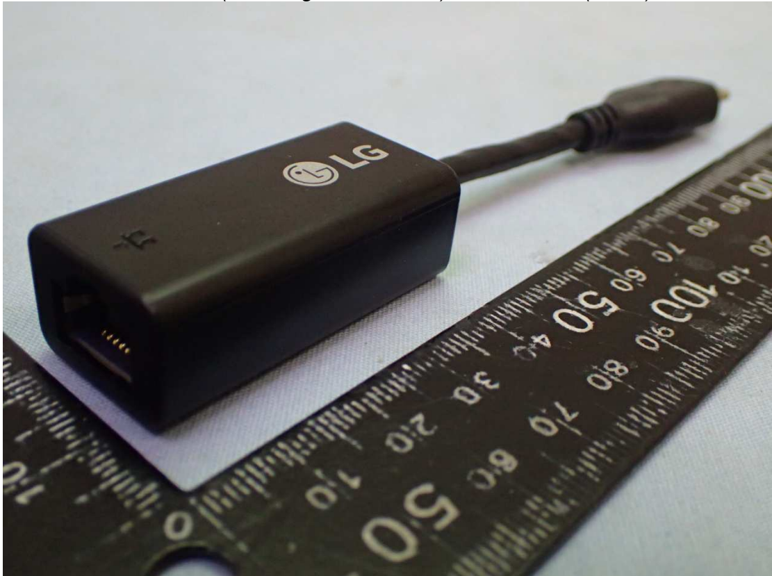
Figure 55 MEC & ARIN (100 Megabit Ethernet), LANGender (Black), Front View
