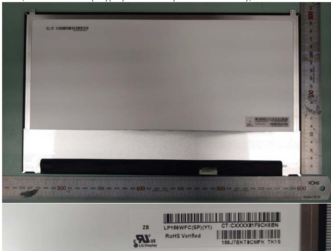
Figure 34 LGD, M/N LP156WFC(SP)(Y1) LCD Panel (Normal Non touch), Back View/ Label View
