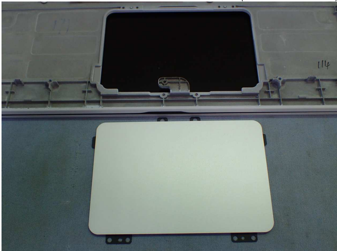
Figure 18 Internal View (Removed Touch Pad)
