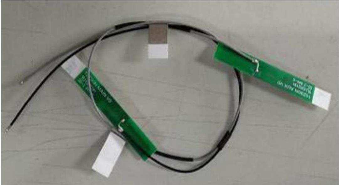
Figure 33 M/N WA-P-LBLB-04-070, WLAN Combo Antenna
