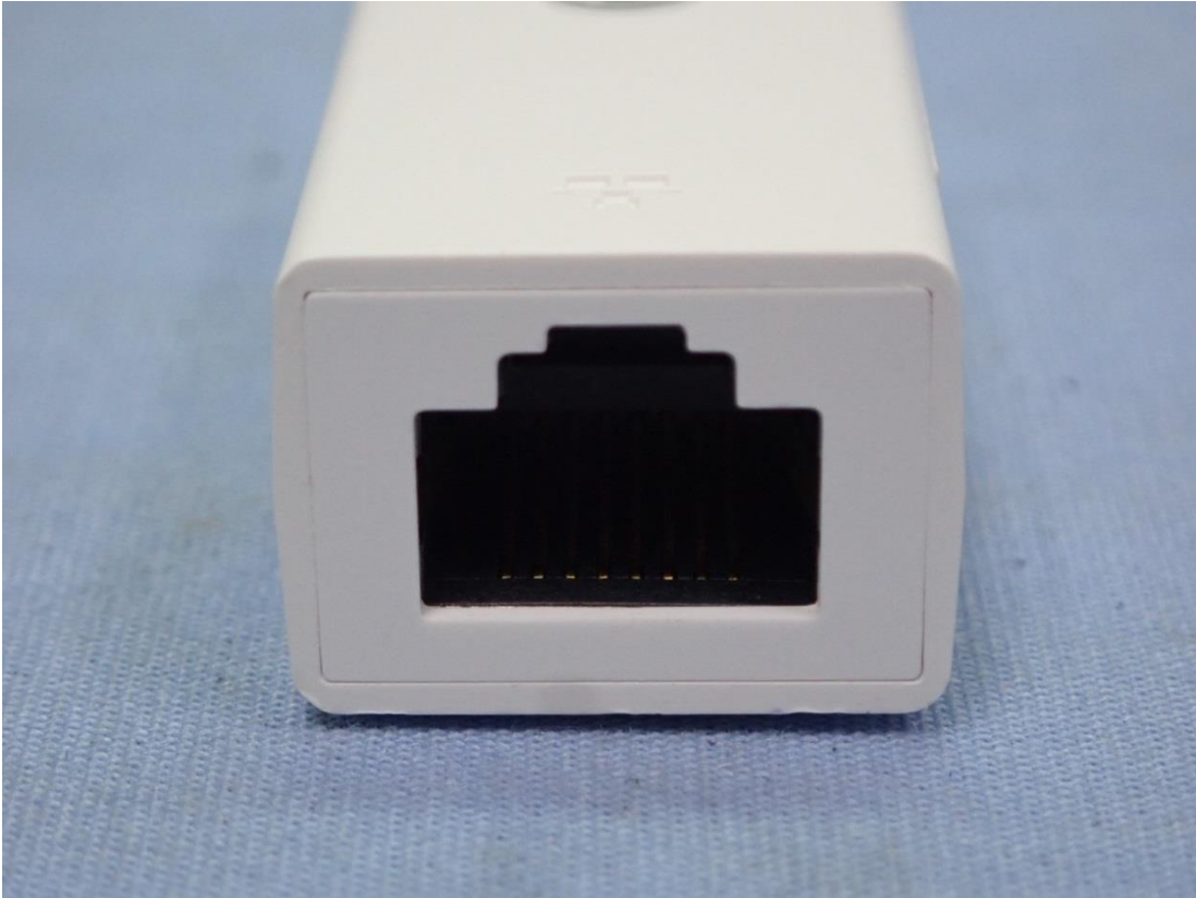
Figure 21 LAN Gender View, Port View
